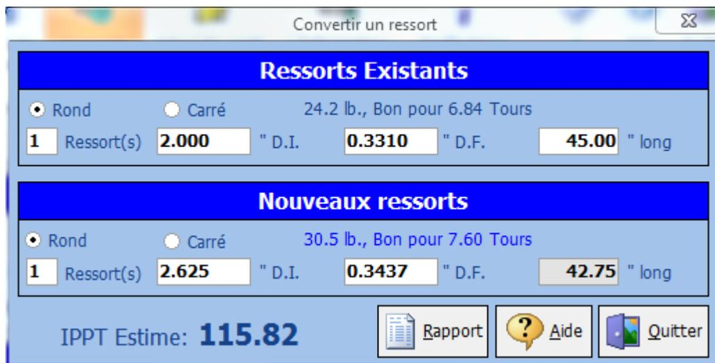
The **TSC** program allows for complete flexibility to all the conditions that you may encounter. You may try to design the new spring by either changing the inside diameter or the wire diameter, or both of them. You may also convert square wire springs to round wire ones. This is very advantageous when you wish to replace existing door spring(s) with a new one, which is readily available in your inventory.
